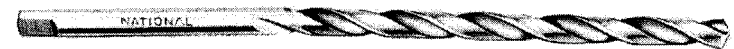
Figure 4-3 Taper-length, tanged, automotive series, straight-shank twist drill regularly furnished with tangs for use with split-sleeve drill drivers. (Courtesy National Drill and Tool Co.)
